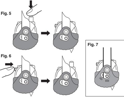
In Fig. 7 note the inscription on the rubber foot. "HH" stands for "Hi-hat" and is the factory set position for the H-2000. For best performance, do not change this setting.
