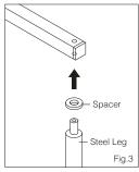
2: Insert the Top of Leg through spacer into the joint hole located underneath the Bar. (Fig.3)
