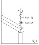
**3:** Screw in Bolt (S)/M10x25 through washer into the top of leg. (Fig.4)
