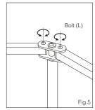
You can adjust the angle of both of the bars with the bolts.
