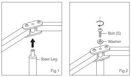
1: Insert the top of leg into the leg bracket of the joint assembly and tighten the Bolt (S)/ M10x25. (Fig.1, 2)
