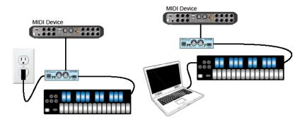
The KMI MIDI Expander is required to send and receive MIDI Data via 5-pin MIDI devices. The MIDI Expander can be used with or without a computer or iPad connected. Power is supplied to QuNexus from the MIDI Expander's power port when the MIDI Expander is plugged into a power outlet. If connected to a computer (or iPad) and a MIDI Expander, power is supplied to the QuNexus from the Micro USB port instead of the Expander.
