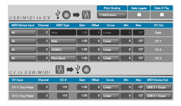
Here you can choose how the QuNexus keys send and receive CV (Control Voltage). QuNexus has 4 possible CV outputs and 2 possible CV inputs (see the CV Manual for the hardware specs).
