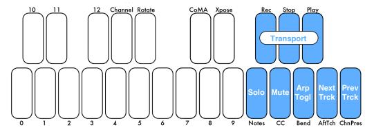
The top 8 keys on QuNexus will control transport, the arpeggiator, track selection, mute, and solo (shown in blue). The other keys (shown in white) can be used for playing melodies. These keys also use Pressure to control modulation and tilt to control pitch bend. The Expression Pedal controls Playback Position. For more information on using this preset with Reason, refer to the QuNexus Symphonix Evolution Quickstart document.
