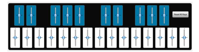
The above window will open. Use the sliders to make adjustments to the sensitivities of specific keys. Move the slider up to make the key more sensitive or down to make it less sensitive.
