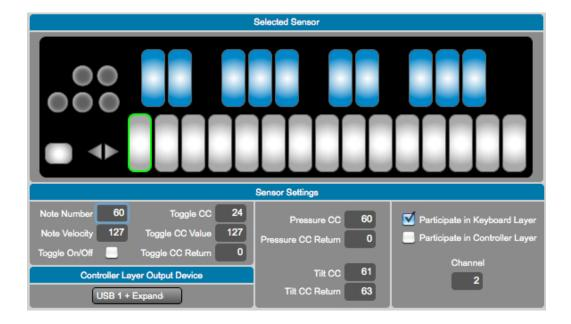
The Controller Layer tab appears next to Keyboard Layer. Here you can assign each key its own additional Note, Toggle CC#, Pressure CC#, and Tilt CC#. Do this by clicking on any key in the image so that it is highlighted with a green border. Then look below the image at the Sensor Settings.
