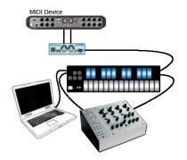
Use Case: This is a good way to play CV with QuNexus, a different hardware MIDI device, and/ or MIDI software on the Computer. This is the most complicated set up but it allows you to do everything the other three scenarios can do above. Ableton Live will be used as the software example in this scenario but you can check for all the same things using different software.
