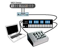
Use Case: This is a good way to control a MIDI hardware device or MIDI software on a computer with an Expression Pedal (or any other uni-polar 0-5 Volt CV source). Ableton Live will be used as the software example in this scenario but you can check for all the same things using different software.
