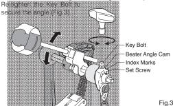
Set Screw Power Finesse The most popular settings are between the "A" to "B" Index Marks. Settings toward "A" offer increased power, and settings toward "B" offer increased finesse. Settings extending beyond that range will be more extreme. For general use, adjust the Set Screw to the center of the "A" and "B" Index Marks on the Beater Angle Cam as shown (Fig.4). Fig.4
